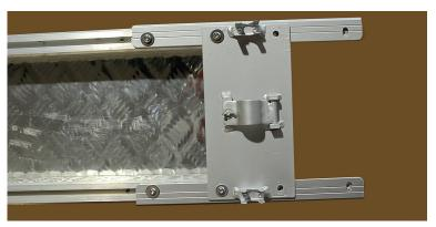
Now connect the base plate to the rails. To do this, use the 2 middle holes so that the plate sits in the middle. There are no washers provided here.
