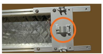
In the next step, be sure to use two people to place the entire running surface with the red-marked fastener on the base.
